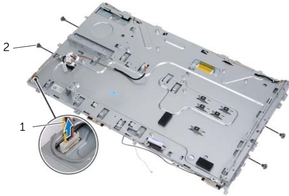
1 converter-board cable 2 screws (4)
